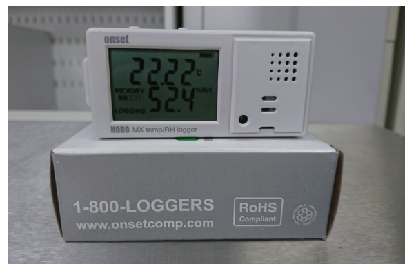
■ 圖 45. 數位式溫濕度計與電子式溫濕度計外觀 Figure 45. Digital and electronic hygrometer & thermometer
