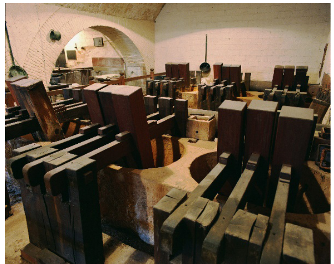
Figure 5. The interior of the paper mill hammers for pulp. Paper Museum Mill. The production of paper was introduced into Europe through Spain in 12th, by the Islamic invaders who had been in contact with China culture, and some years later from Italy. (Source: Eusebi Casanelles)
