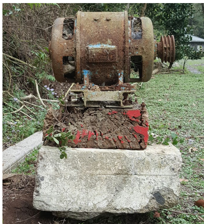
Figure 2. Shanping - excavated 3 phase 5kW generator with wooden anti-vibration mat and concrete base.
