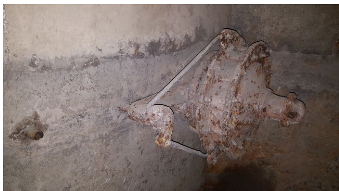
Figure 3. Shanping - excavated and cleaned horizontal axis open flume Francis turbine.
