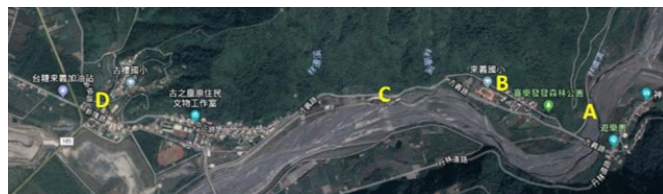
Figure 4. Distribution of Er-Feng Irrigation Canal System along the Linbian River. A: Water inlet tower; B: Canal waterway outlet and lateral overflow weir (overflow channel); C: Tunnel waterway outlet; D: Water diversion structure (Map data ©2019 Google).
